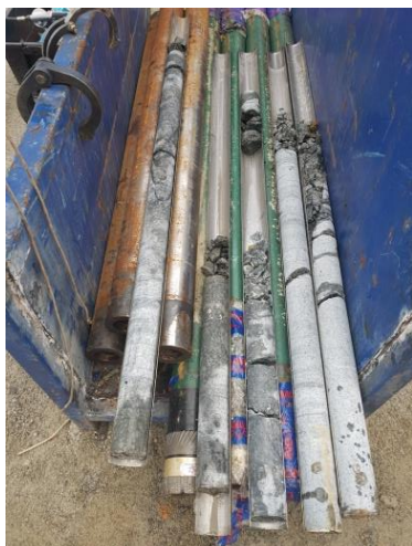
Typical core retrieved using HMLC triple tube barrels with combination of surface set and impregnated bits (series 10) 1.5m sample tubes
