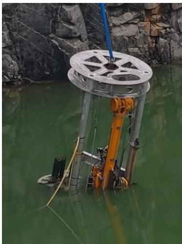
Landing and drilling greater than 20deg during endurance testing
